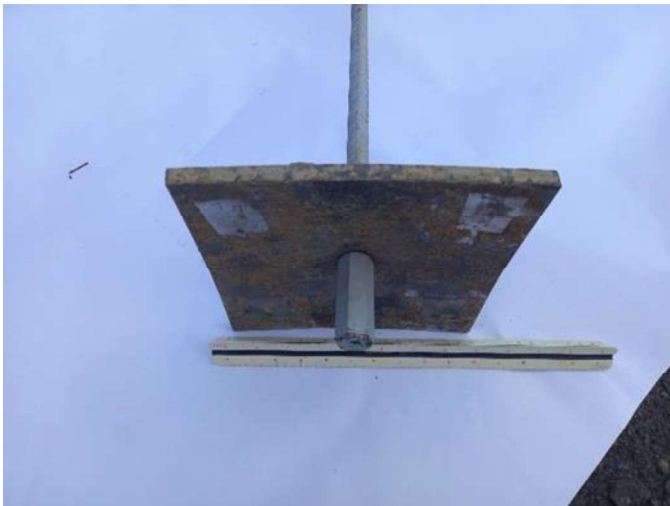
Figure 18. Deformed Anchor 14 following exhumation
